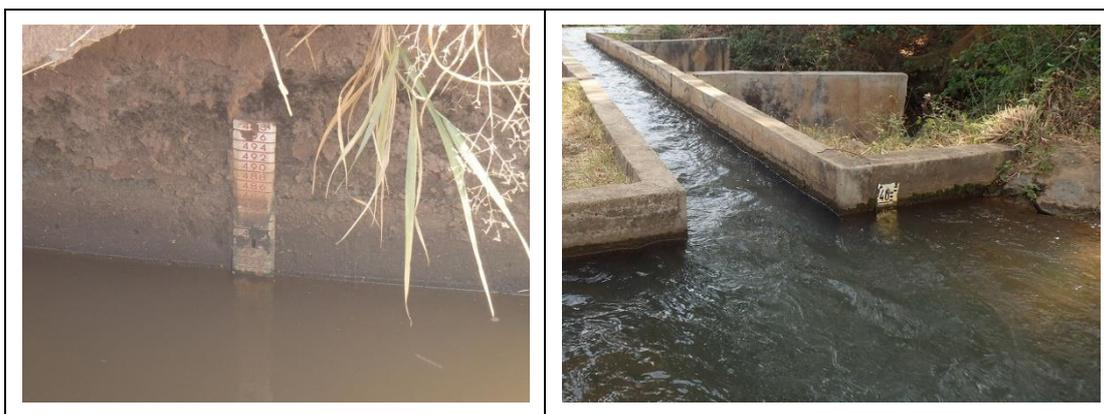
**Figure 4-15: Installed water level gauge.**
