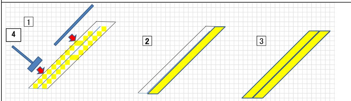
For Good compaction of Side-wall, Wooden compacting tools are used instead of vibrator. Concrete hit hard 3 times per location by tools to release air. Sub-step 2 and 3 shall be done in short time for a good quality of concrete wall/ base.
