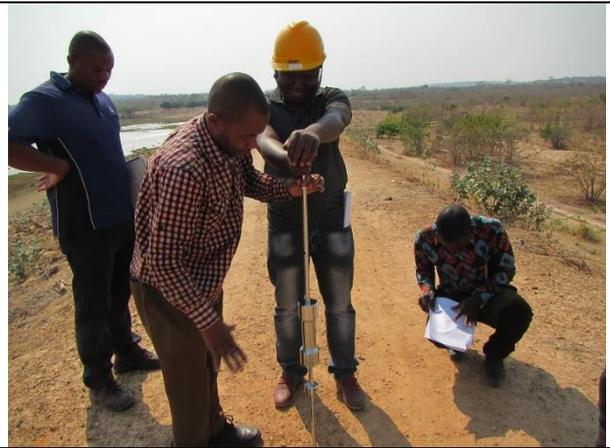
9. After step-8 is complete, Hold the device up-right then continued for the 4th 0.1m layer "0.3m – 0.4m" (225)
