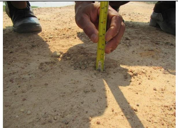
16. (continued) Penetrated depth by Nd=50 was measured as 6.6cm and also recorded for Layer “0.9m – 1.0m” (2262) Test can be continued, if Nd=50 NOT reached.
