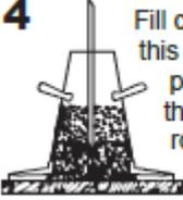
Fill cone <sup>2</sup>/<sub>3</sub> full by volume. Rod this layer 25 times with rod penetrating into, but not through first layer. Distribute rodding evenly over the entire cross section of the layer.</p>                                                                                                                                                          |
