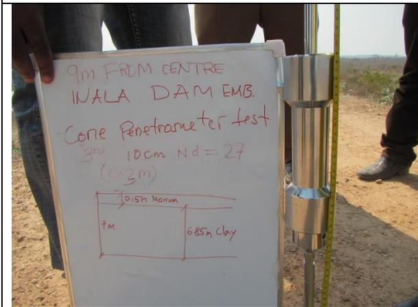
7. In the same manner the penetration of 3<sup>rd</sup> 0.1 m conducted, the number of hitting was 27, thus recorded as Nd=35 for layer “0.2m – 0.3m” <sup>(2234)</sup>
