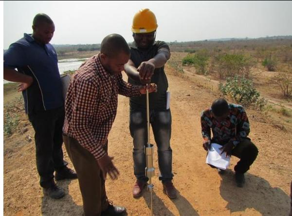
Checking the 1<sup>st</sup> “10 hits (Nd=10)” at Site-2<sup>(2216)</sup>
