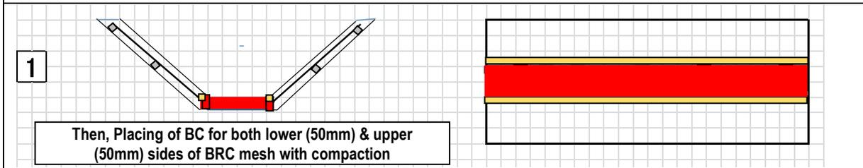
**Placing of Base Concrete (BC) with compaction**
