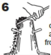
Remove the excess concrete from the top of the cone, using tamping rod as a screed. Clean overflow from base of cone.</p>                                                                                                                                                                                                                                            |
