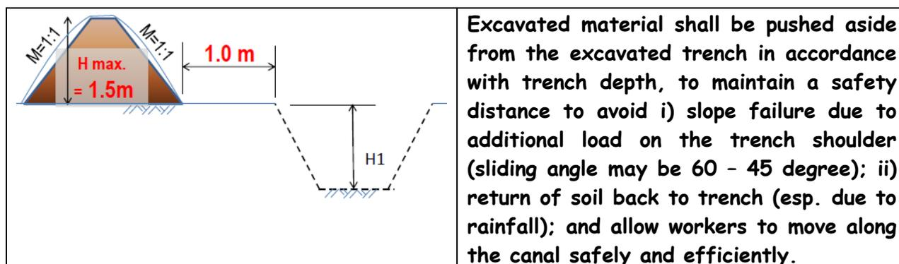
Excavated material shall be pushed aside from the excavated trench in accordance with trench depth, to maintain a safety distance to avoid i) slope failure due to additional load on the trench shoulder (sliding angle may be 60 - 45 degree); ii) return of soil back to trench (esp. due to rainfall); and allow workers to move along the canal safely and efficiently.
