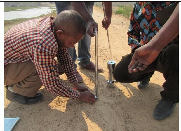
8. After the 3<sup>rd</sup> layer test, Handle, Weight, Rod for weight and joint shall be removed, remaining Cone+ Rod-1 still, using tools, then one additional rod to be added to Rod-1 <sup>(2238)</sup>
