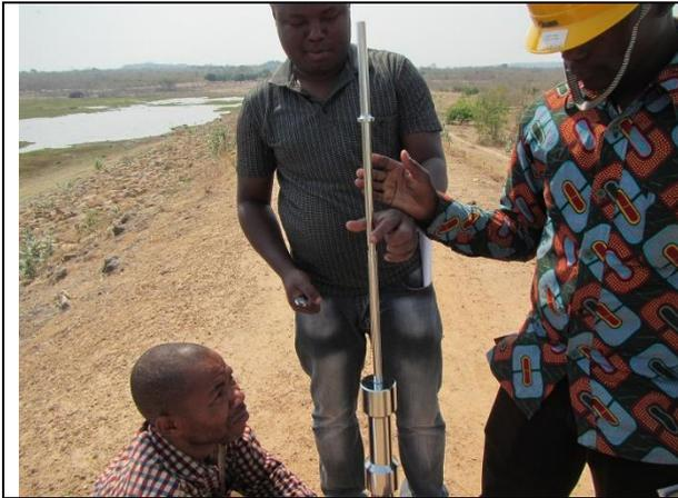
8. (continued) After one rod is added to Rod-1, confirm rod and other parts are tightened firm using tool up to handle (224)
