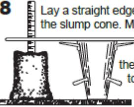
Lay a straight edge across the top of the slump cone. Measure the amount of slump in inches from the bottom of the straight edge to the top of the slumped concrete at a point over the original center of the base. The slump operation shall be completed in a maximum elapsed time of 2 1/2 minutes. Discard concrete. <b>DO NOT</b> use in any other tests.</p> |
