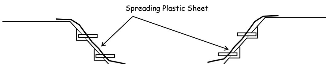
Note: In case of using the plastic sheet, filling joint sealer to the groove is not necessary to the lining joint groove.
