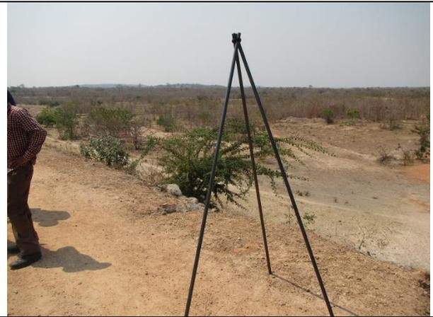
17. (continued) If penetrated depth is very deep and removal of device by hitting upward is difficult, a tripod with hook, rope and pully shall be used for as an aid (236)
