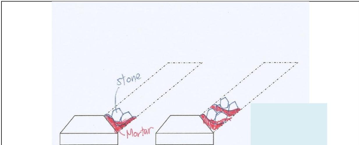
Starting from the Bottom, placing mortar at bottom & behind of the wall then put stones on top to make sure mortar is well jointed with stones near by
