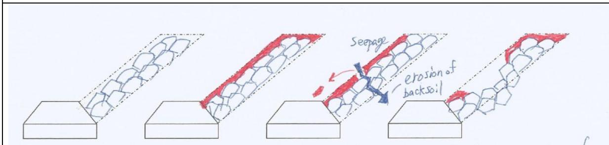
Placing stones only first without any joint mortar between and around stones. Then only plastering on the surface.
