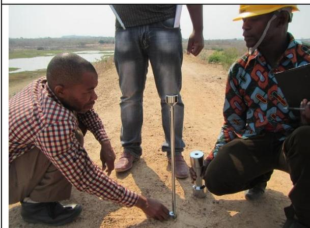
8. (continued) After one rod is added to Rod-1, confirm rod and other parts are tightened firm using tools <sup>(2241)</sup>
