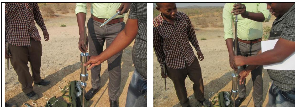
Initially, the device is assembled with order of 1 -> 2 -> 3 -> 4 -> 5, using tools for tightening the devices and rods, for accurate test, without losing any parts when device pulled-up after test.
