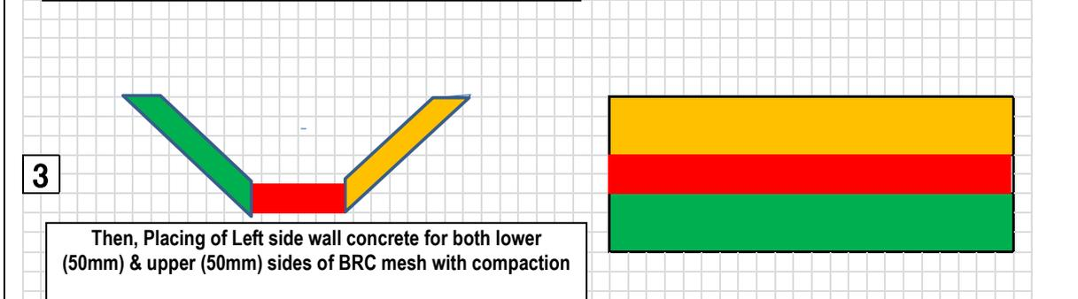
**Placing of Side-walls Concrete with good compaction**
