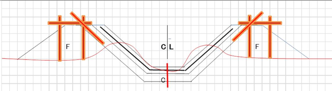
Alternative setting-out by installation of a pair of hinges/ batter boards showing slanted excavation lines and elevation of the embankment (earth-filling)/ canal top
