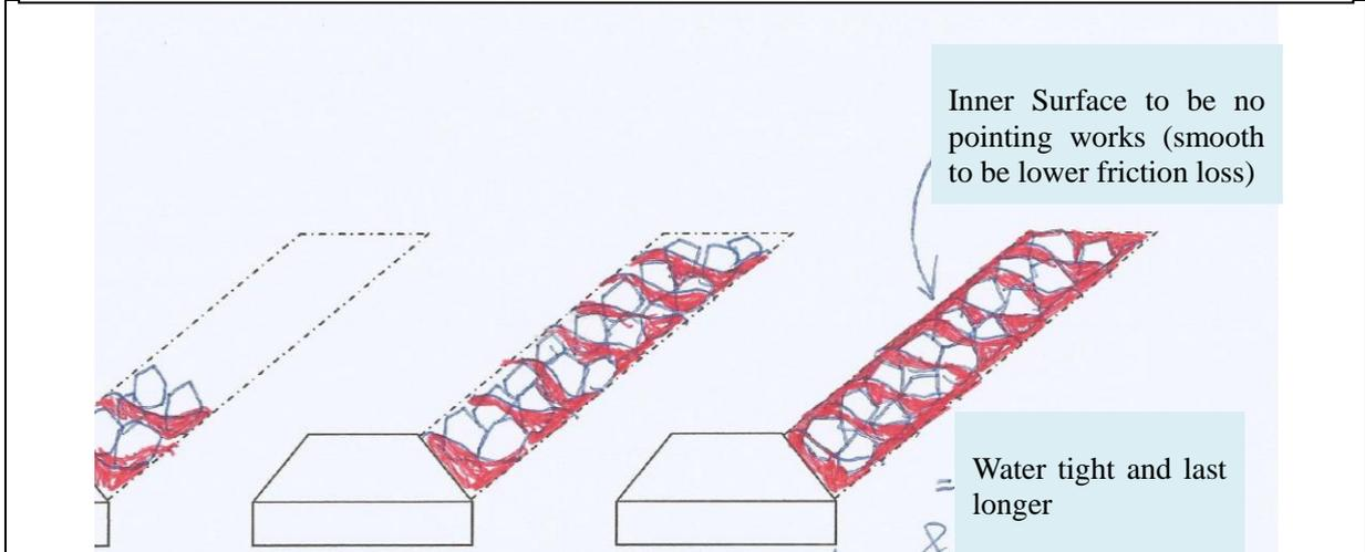
then build toward upward. Finally finishing with plastering without pointing
