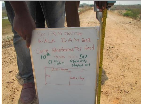
16. For the 10th 0.1m layer, at Site-2, the number of hitting reached to Nd=50. And recorded Nd=50 for “0.9m – 1.0m”. The Test shall be STOPPED if Nd=50 is reached. (2261) - SC1 (2261)
