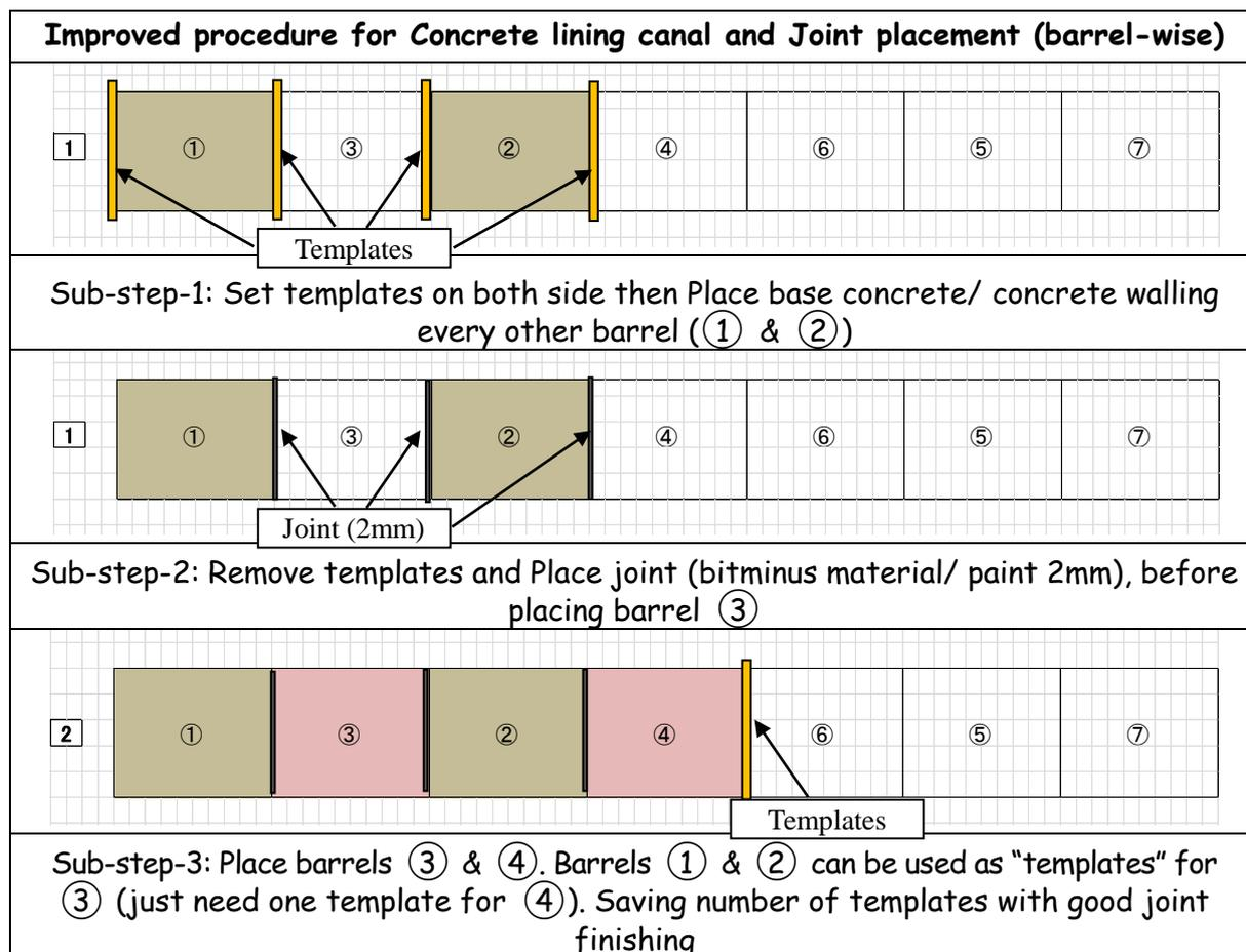
Especially for a small scale canal with concrete lining (Bottom width  $\leq 1.0\text{m}$ ), in cross-sectional wise the following procedure shall be applied for each barrel as shown on next page, i.e. placing BRC (R6 x 150 x 150), using mortar spacer block (50mm x 50mm x 100mm, Cement: Sand ratio = 1:2, spacing of 1 block/  $\text{m}^2$ , tied with BRC by wire) for keeping specified cover underneath the BRC mesh, and as a part of formwork for the base concrete.
