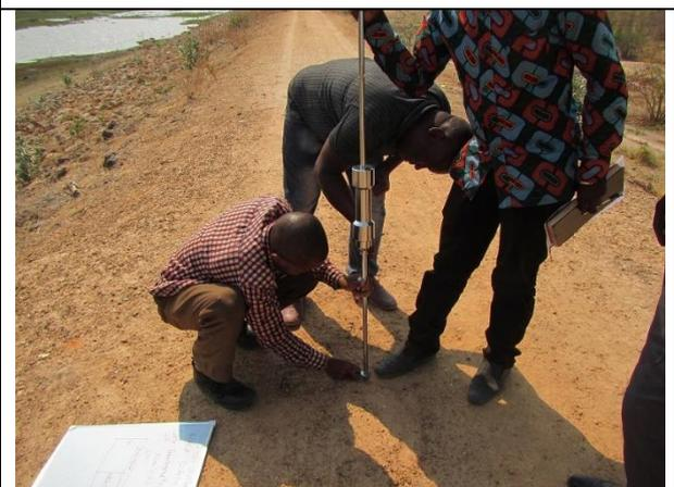
8. (continued) By adding one rod to Rod-1, enable for testing up to 1.0m depth <sup>(2241)</sup>
