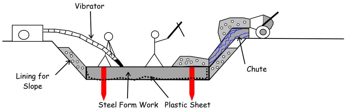
➤ Compacting Lining Concrete using Vibrating Plate with Spikes:
