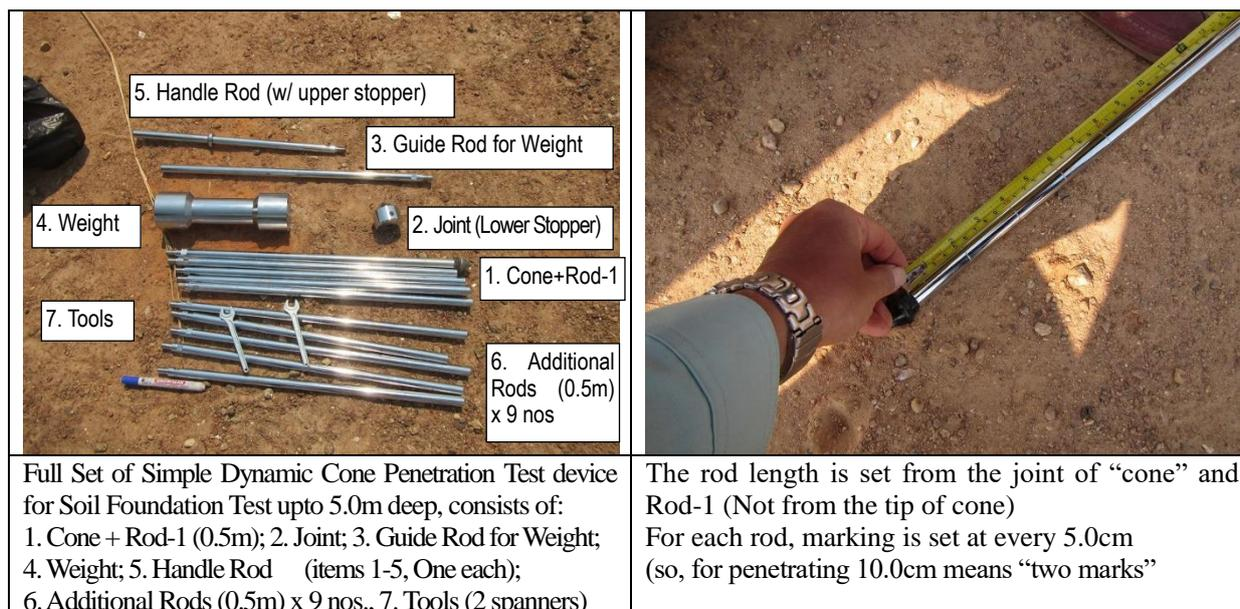
Full Set of Simple Dynamic Cone Penetration Test device for Soil Foundation Test upto 5.0m deep, consists of:
