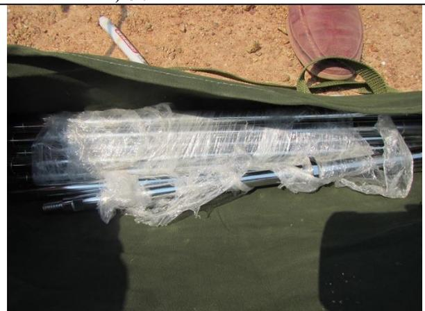
20. Rod-1 w/ cone, Handle, Rod for weight and additional rod, removing soil completely, then pack (236)
