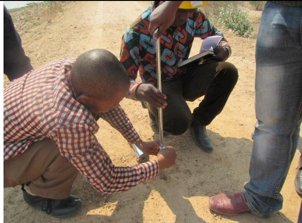
14. After completion of the 8th 0.1m layer, another additional rod to be added, enable for testing up to 1.5m depth, as same manner as Step-8 (2255)
