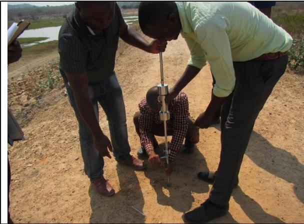
17. If Test is STOPPED and necessary records are made, the device shall be removed by hitting the "Handle Stopper" upward. If penetrated depth is deep, remove the additional rods and re-tightened for easy remove (236)
